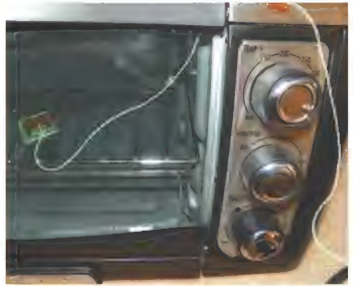
Figure 7. Thermal sensor attached to PCB in the oven.
